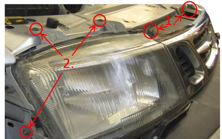
7. If vehicle are equipped with headlight vipers, first remove the washer hose from the viper blade arm and then remove them by folding up the plastic cover (1.), removing the 8mm hex nut (2.) located underneath and then wiggle it a bit at the same time as you pull it of the axle.
