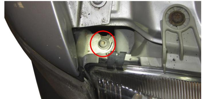
6. Remove the front grille by pressing the metal clips (1.) and then lift grille upwards. Remove headlights by disconnecting the electrical connector (info below), removing the 3 screws (2.) that attaches them. Lift free from tab in rear area and pull forwards out of the car.
