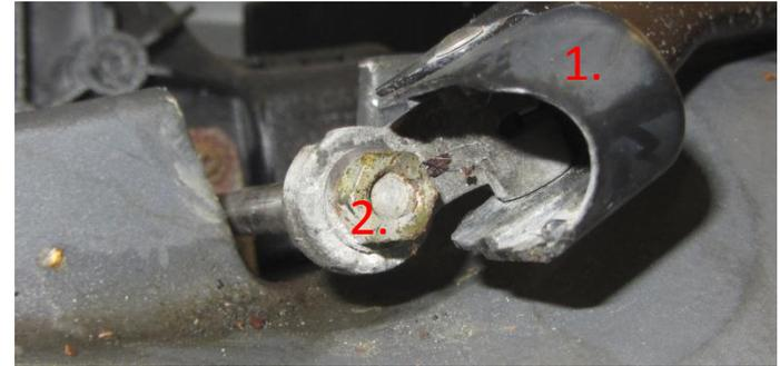
8. Remove the bumper from car by removing the 2pcs 16mm hex screws then hold out the rear part of bumper so it comes loose from the inner fenders and then move the bumper forward until it's a few centimeters ahead of car and in this position remove the ambient temperature sensor from the lower grille in the bumper cover.
