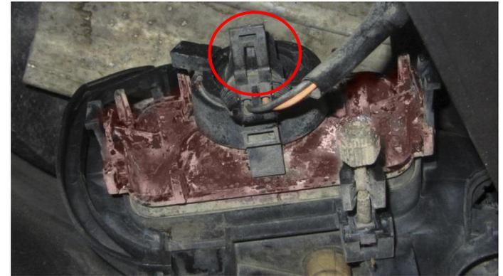
5. Remove front indicator lights by removing the 1 screw that attaches it to the headlight from the top. Then pull the indicator light forwards and remove the electrical connection.
