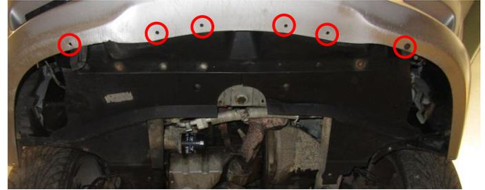
2. Remove the 1pcs screw on each side of vehicle that holds the bumper to the inner fender.
