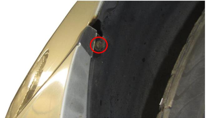
3. Remove the 1pc screw on each side that attaches the plastic radiator protection to the inner fenders.
